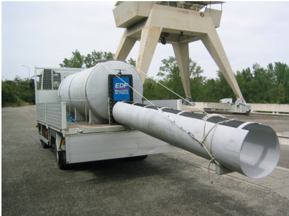
Figure 3.16: Truck of the Garonne River trap & truck scheme. The fish are transported 200 km downstream and released below the lowermost Golfech dam. (Photo: Marq Redeker)
